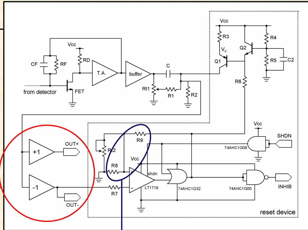
(2) Adjust ToT comparator thresholds
