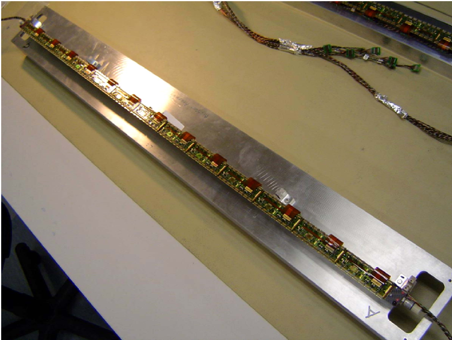
13 modules mounted on one stave with carbon-carbon support structure and cooling pipe
