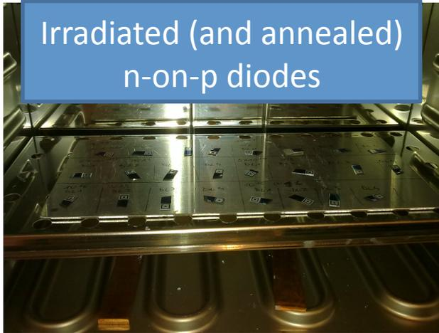
Irradiated (and annealed) n-on-p diodes
