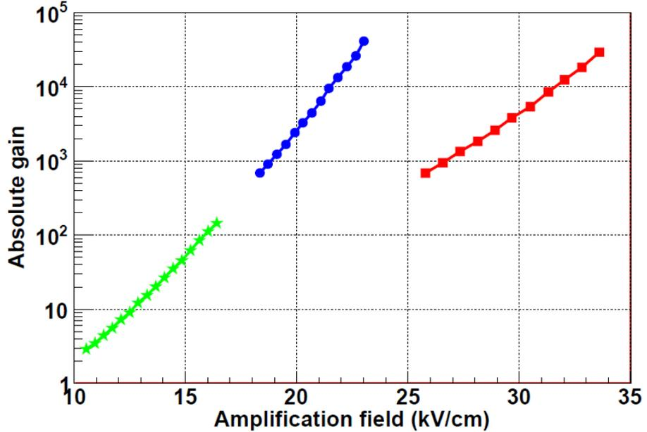
Amplification gap = 256 μm
