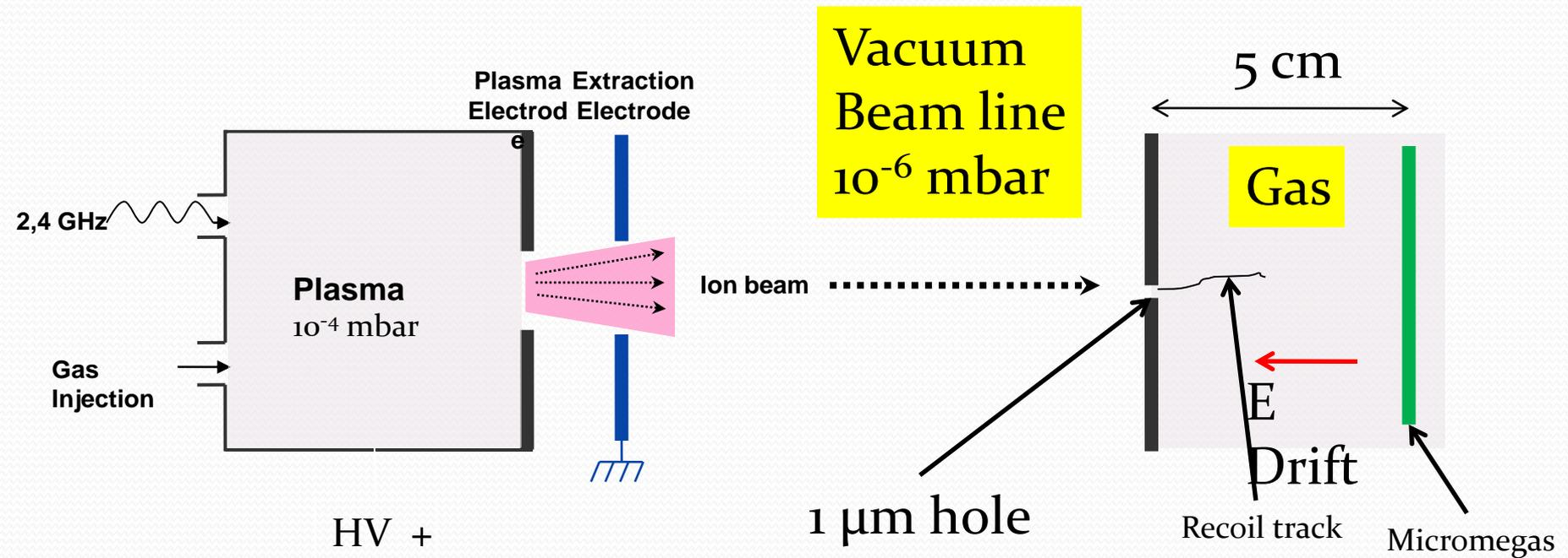
Ions are injected through 1  $\mu\text{m}$  hole inside gas chamber
